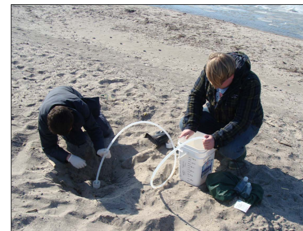
Purging the piezometer water
