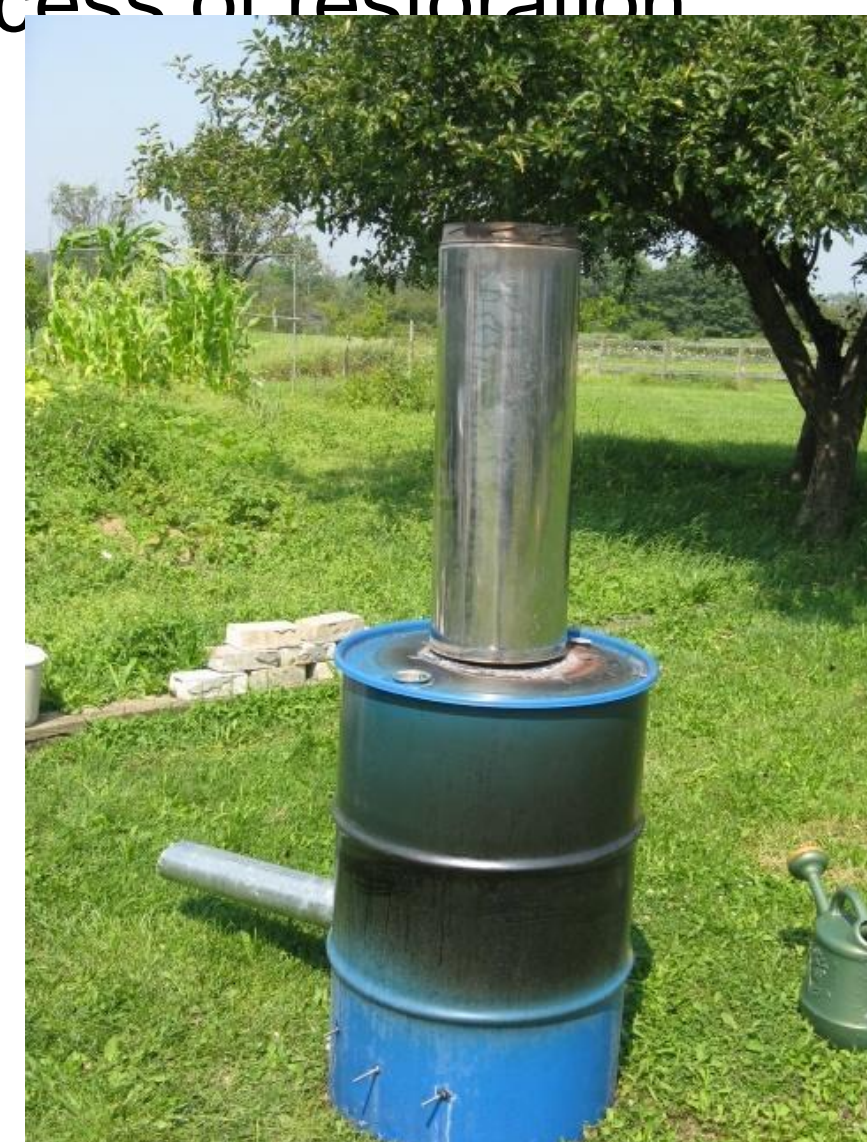
Biochar stove constructed by Rob Diemair using a Barrel and stove pipe fittings. Optimally it burns at 200°C
