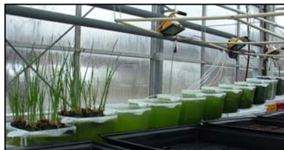
The four-step in-house gravity flow through system (Gole 2009).
